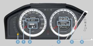
**Trip odometer.** To measure distance the car has two independent trip odometers T1 & T2 always running.
